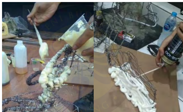
Lampiran 3. Proses penambahan material Polyurethane .
