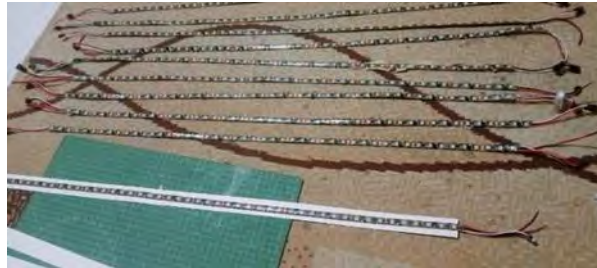
Gambar 2. 36 Proses perakitan LED WS2812b
