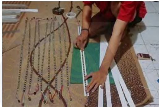
Gambar 2. 37 Proses perakitan LED WS2812b
